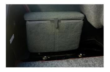
2) Remove the trunk CD changer if equipped a) Remove the fabric cover by pulling up and over the top of the CD changer.
