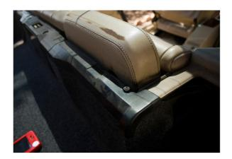
14) Remove the screws holding the plastic trim piece in place. Then lift out the trim piece.
