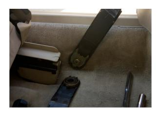
16) Remove the cover for the passenger side seat belt swivel. Remove for rear side wall trim romval then replace.
