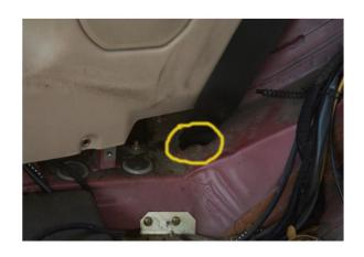
17) Unbolt rear seatbelt mounting bolt. Once the rear sidewall trim is removed, replace the mount.
