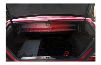
6) Remove the large center trunk liner a) Removal will require pulling it out and manipulating it to squeeze out
