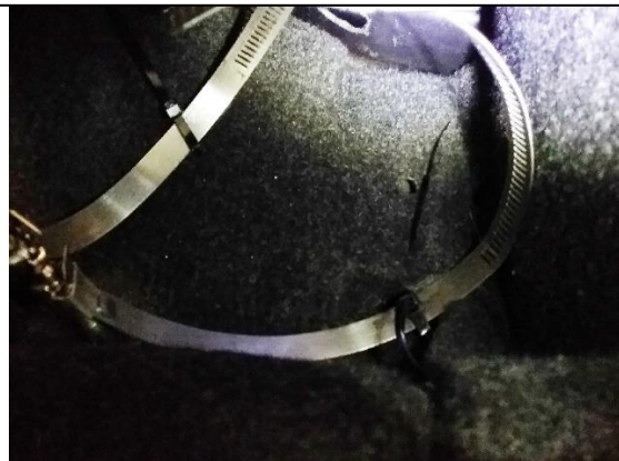
View of clamps connected to the zip ties with the plate installed behind the carpet inside the trunk
