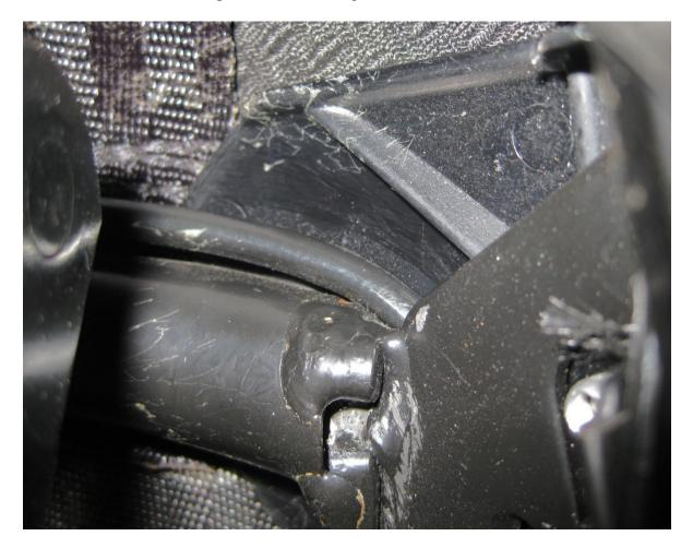
The plates are attached from the top with 2 rivets. To access these rivets requires removing/loosening the fabric from the top, which requires drilling out many rivets. This is not a solution I'd like to pursue.
