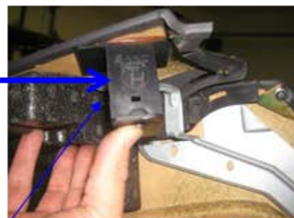
The block is glued to the underside of the top of the side panel. There is a yellow anchor at the bottom of the block that holds the panel down to the metal body work (not shown).
