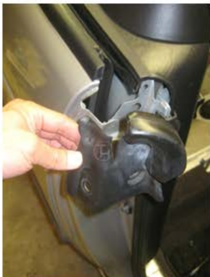
Remove the upper corner seal by lifting straight upwards.
