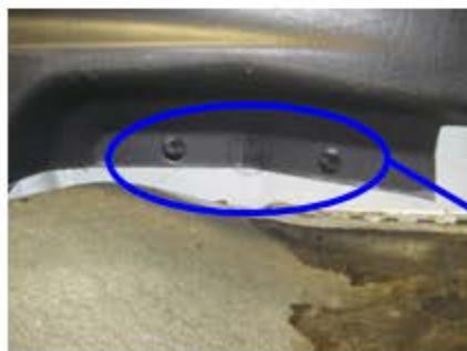
There are 2 plastic quarter turn fasteners along the bottom of the side panel, 1 more at the bottom rear & a torx at the upper rear.
