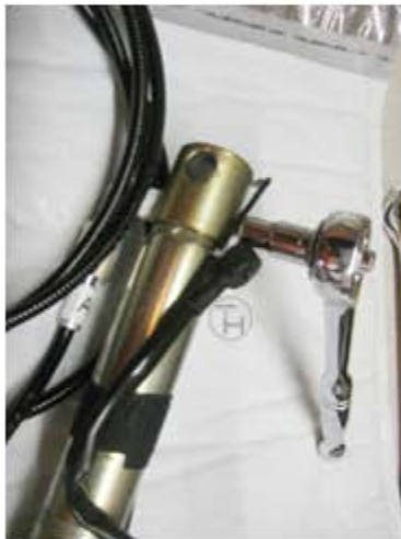
Remove bottom wire with T8 & side with 4mm socket.
