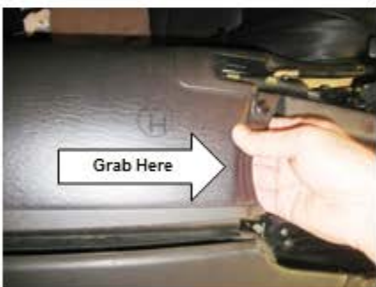
The interior side panel is about ready to be removed. There is one more clip located underneath the top rear portion of the side panel that is tricky to break loose.
