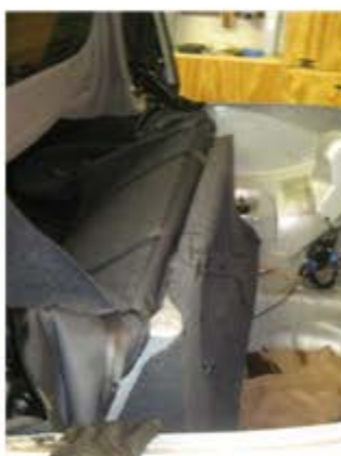
Flip the trunk liner portion of the bag into the rear seat area
