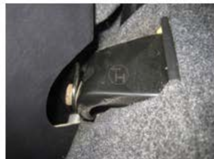
Access to the bolt head is a bit tight, use a ratcheting wrench if available.
