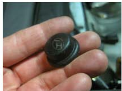
Lift the carpet back & turn the valve counter clockwise to release the hydraulic system
