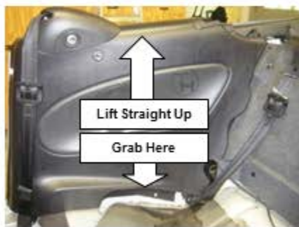
Lift straight up to pop the fastener loose.
