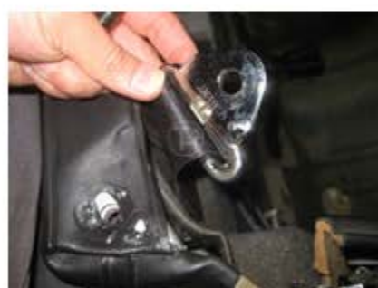
Note the bottom of the plate has a locator pin.
