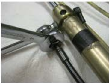
Use a 14mm wrench to tighten the line.
