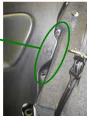
Use a torx driver & pull the screw in the upper forward rear side panel.
