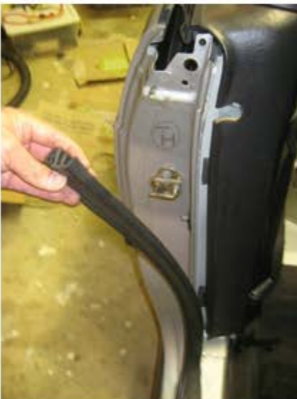
Pull the gasket off - it simply pulls off. All the way down and off...
