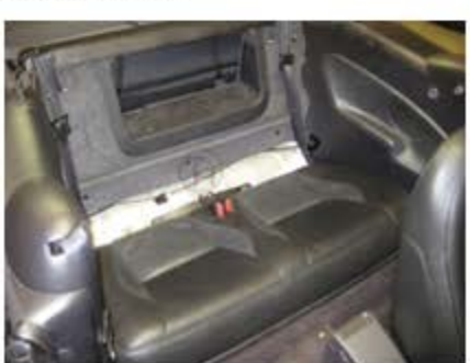
Remove the rear seat back.
