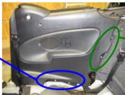
There are 2 plastic quarter turn fasteners along the bottom of the side panel, 1 more at the bottom rear & a torx at the upper rear.
