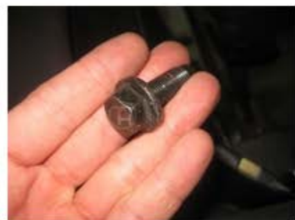
Remove bolts with 16mm socket.
