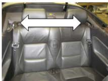
Locate both rear seat belt brackets.
