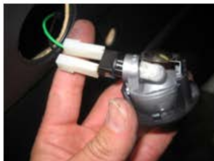
Gently pry it out with a small flat head screwdriver or a scraper.
