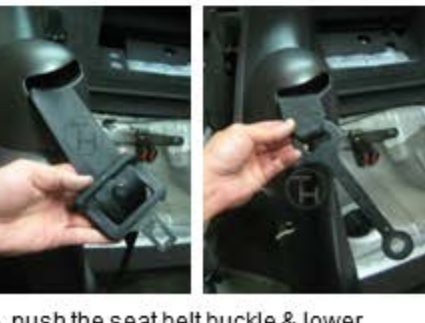
Once you've broken the side panel loose, push the seat belt buckle & lower bracket through the slot in the hump.
