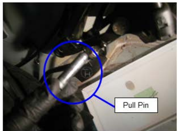
Pull the pin the clip was holding in.
