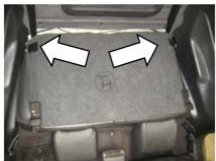
Lay the rear seat back down & locate the 18mm bolts at either end of the seatback base.
