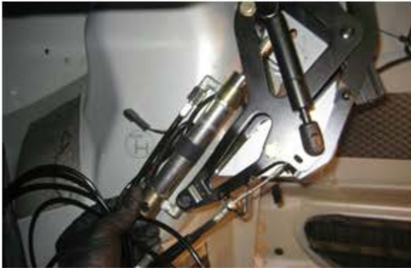
Remove the cylinder & note orientation.
