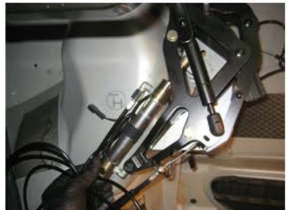
Reinstall the cylinder.
