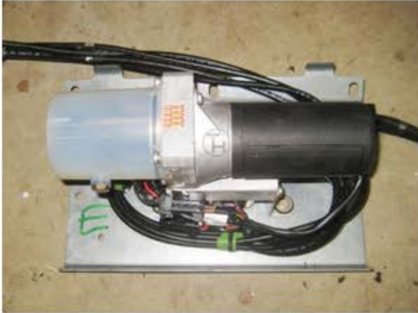
Set pump aside with cut lines still attached.
