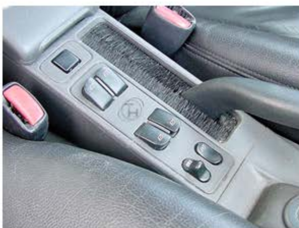
Turn on your vehicle and hit the switch. Cycle the top open and closed 5-10 times.
