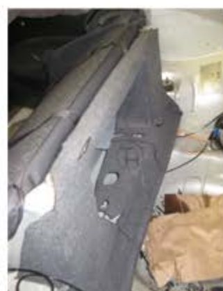
There is an additional liner surrounding the pump area.
