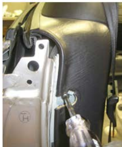
Use a torx driver & pull the screw in the upper forward rear side panel.
