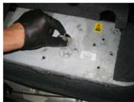
Lift the carpet back & turn the valve counter clockwise to release the hydraulic system
