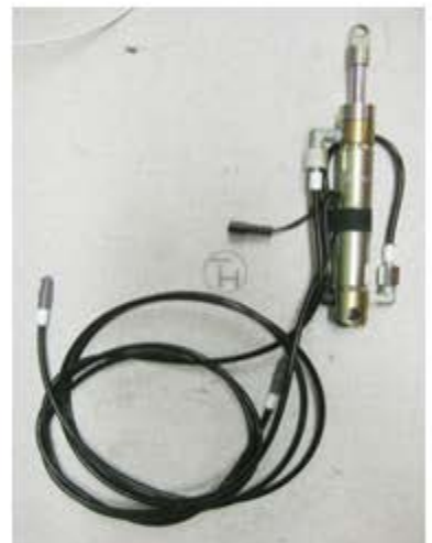
Install line A, X, and the wire. Note: Refer to diagram on pg. 3 for lines & corresponding cylinders. Tape line down the same way as the old one was.
