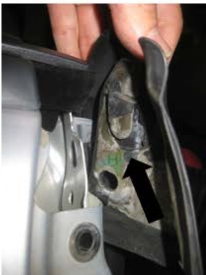
Note there is a hook stamped into the plate backing of the corner seal - you must lift straight up to remove.
