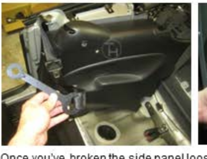
Once you've broken the side panel loose, push the seat belt buckle & lower bracket through the slot in the hump.
