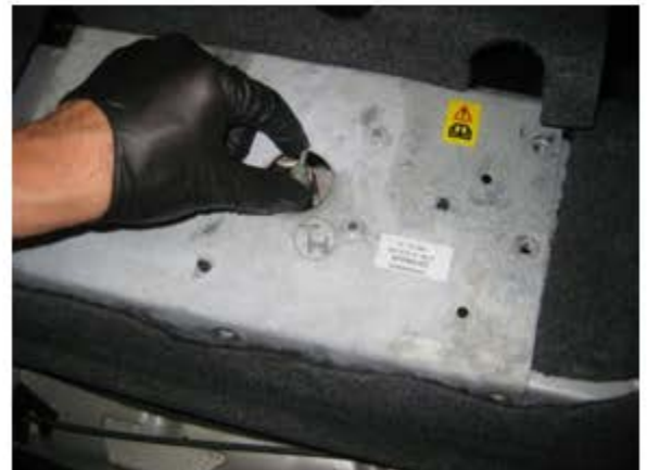
Close the hydraulic release.
