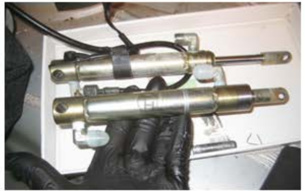
Compare new lift cylinder to old one & note routing of lines, wire, & how its taped down.
