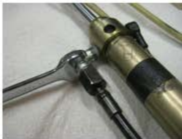
Use a 12mm wrench to hold the lower line mount.
