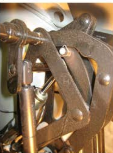
Remove the upper clip and remove pin.
