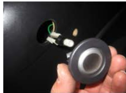
Remove the cover from the light.
