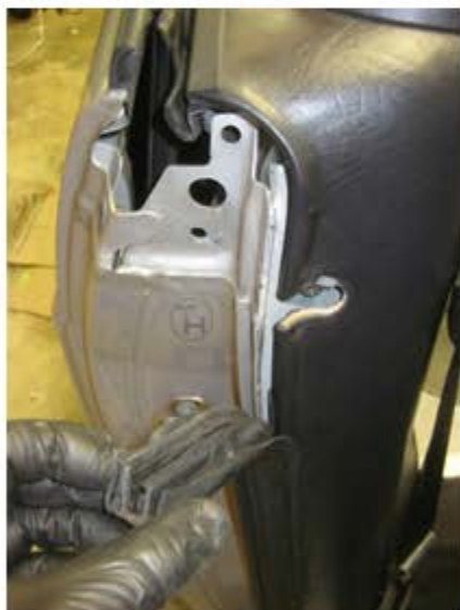
Pull the gasket off - it simply pulls off. All the way down and off...
