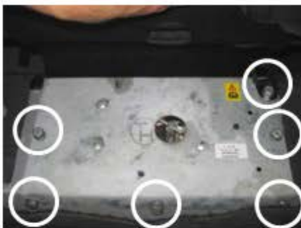
Go ahead & remove the 6 bolts holding the hydraulic pump plate down. Note the orientation of the buckle.
