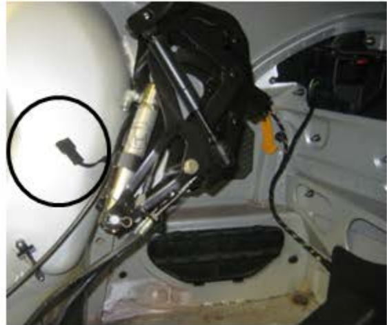
Unplug the wire leading to the cylinder.
