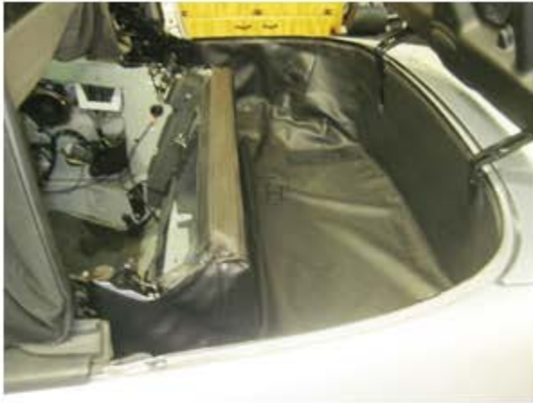
Set the soft top bag and carpeted seat back section into plate.
