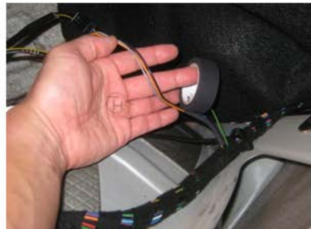
Re-Wrap with new friction tape.
