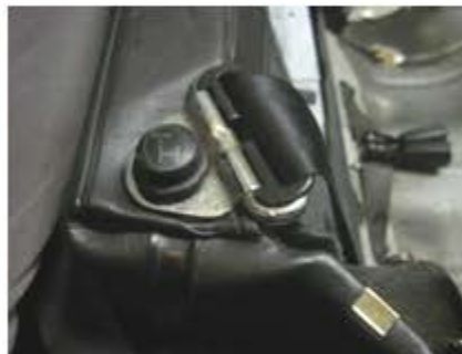
Pop the bolt cap off with a flat head screwdriver.
