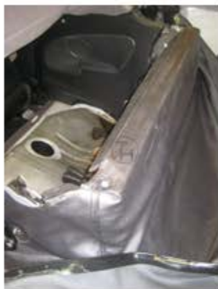
Bag on seat back structure
