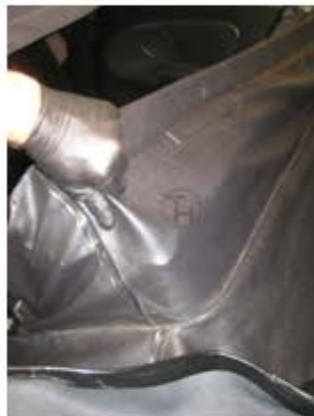
Pull bag up off the structure & bunch the mtrl. forward. Watch the sides of bag still attached to vehicle towards the front as you can tear it.
