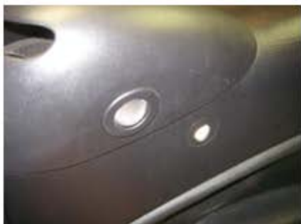
Locate the light in the seat belt hump.
