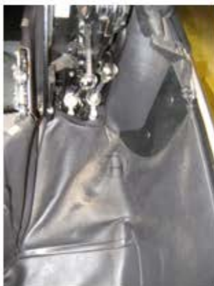
Note plastic plates on either side with 2 fasteners. You don't have to remove them but be careful when moving bag as it can tear here.
