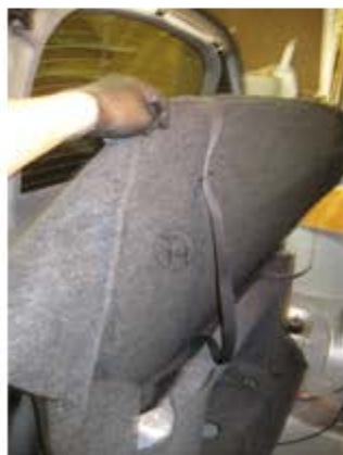
Pull it out from trunk. It has a hard liner in it so it's a bit unwieldy.
