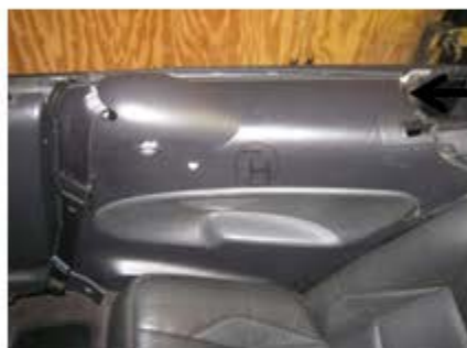
The interior side panel is about ready to be removed. There is one more clip located underneath the top rear portion of the side panel that is tricky to break loose.
